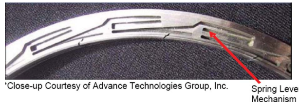
Fig. 2 Photograph of a hybrid brush seal (close up of pad and elastic supports)
